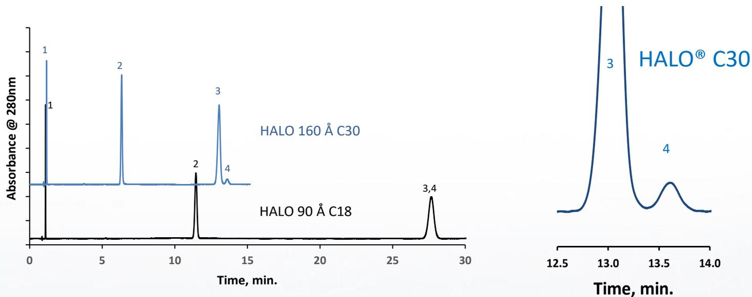
Column format: 2.7  $\mu\text{m}$ , 4.6 x 150 mm
