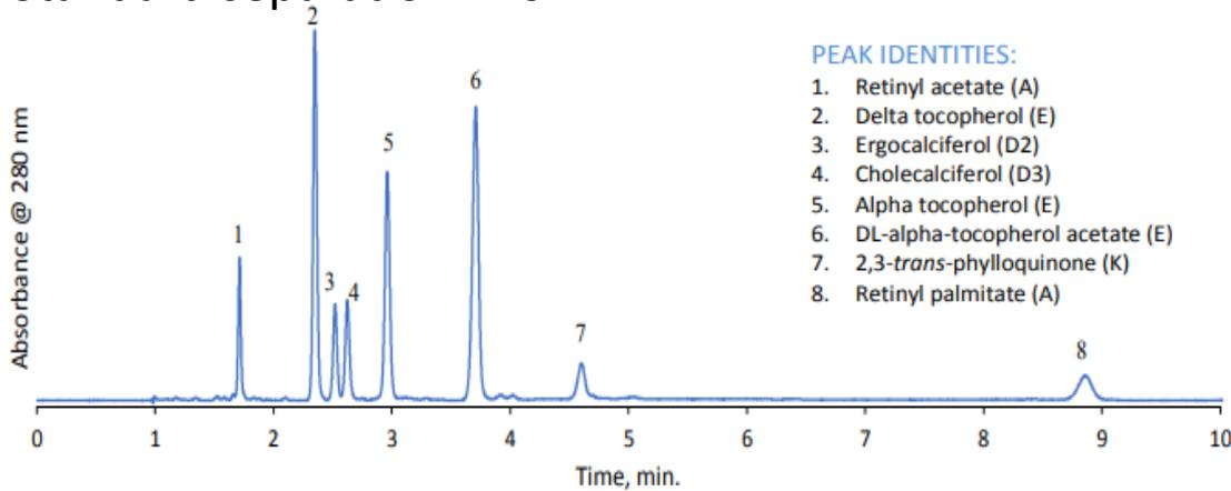
**Analytical Column:** HALO 160 Å C30, 2.7 µm, 4.6 x 150 mm
