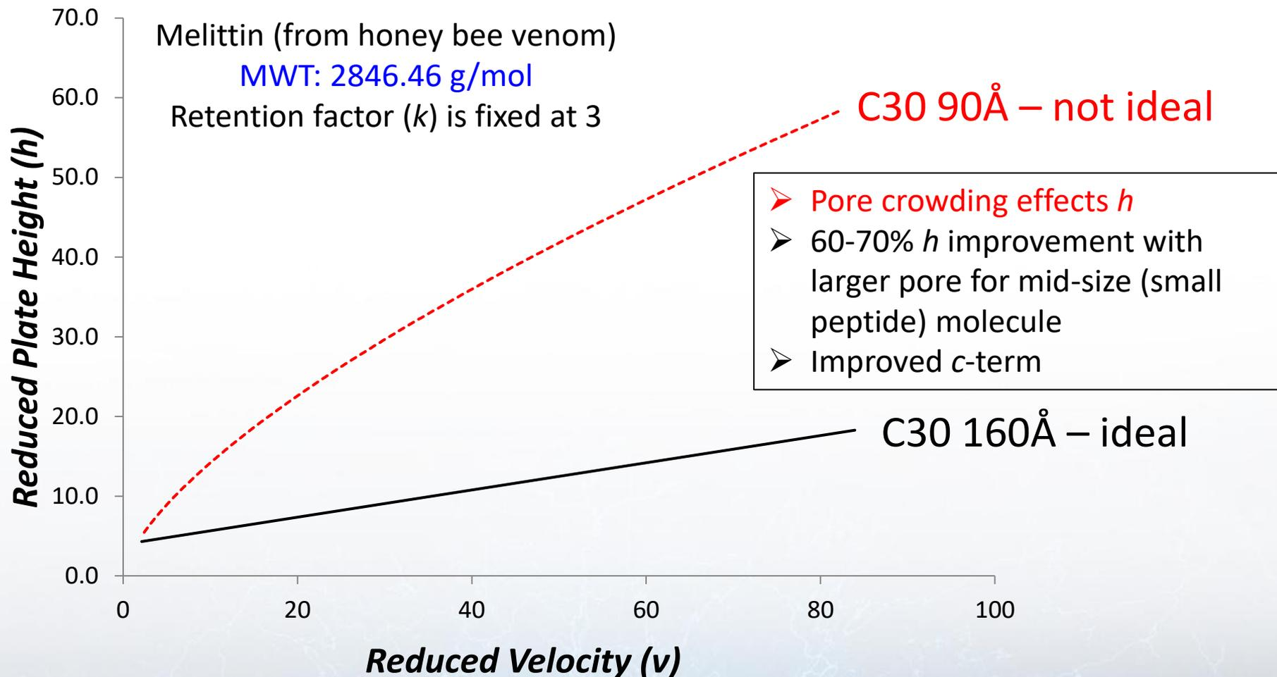
Column: C30 90Å and 160Å, 2.7  $\mu\text{m}$  dp, 50 mm x 4.6 mm
