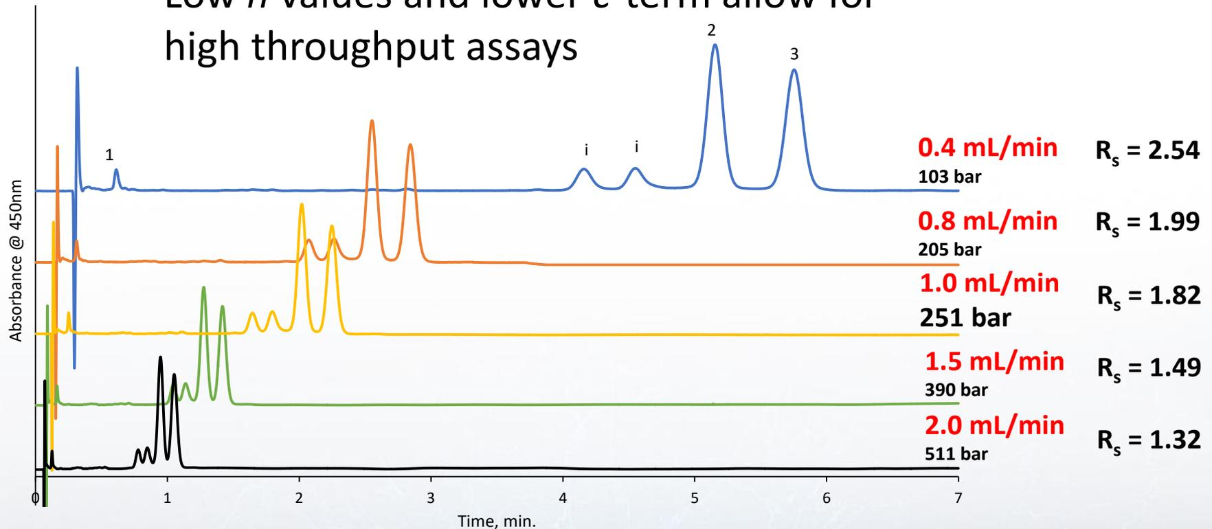
Column: HALO 160 Å C30, 2.7 μm, 2.1 x 50 mm
