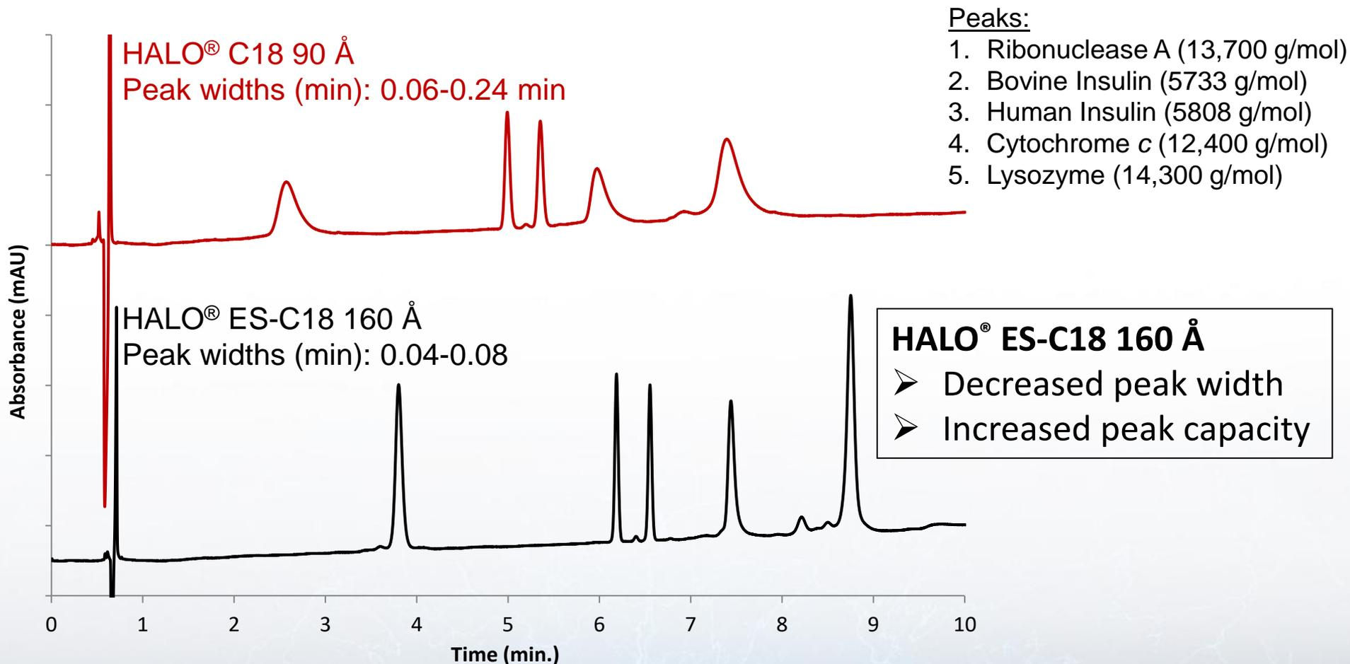
Columns: 2.7  $\mu\text{m}$   $d_p$ , 100 mm x 4.6 mm HALO C18 90 Å pores and HALO ES-C18 160 Å pores;
