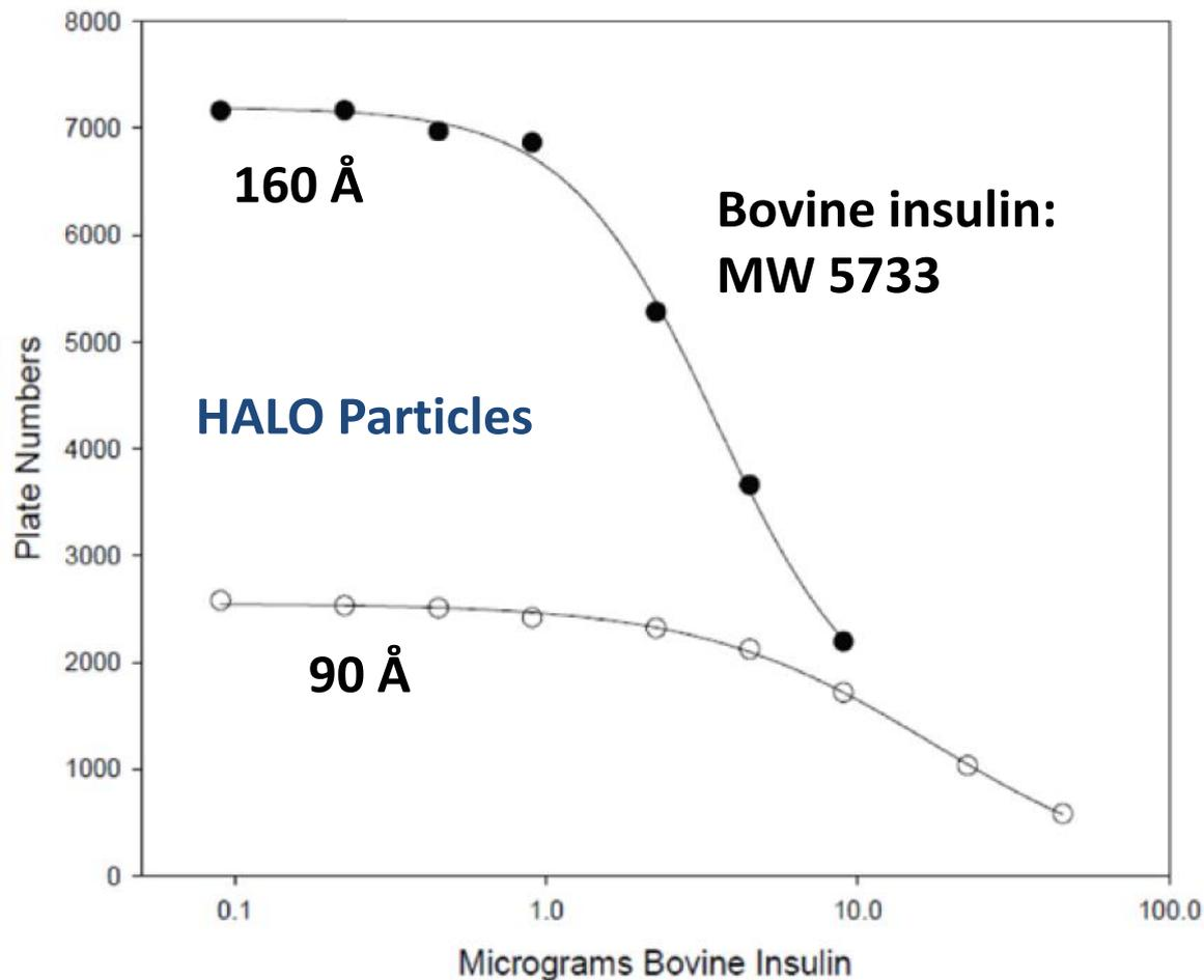
High efficiency is the key to high resolution and peak capacity; a larger pore particle is needed for high efficiency with bovine insulin.
