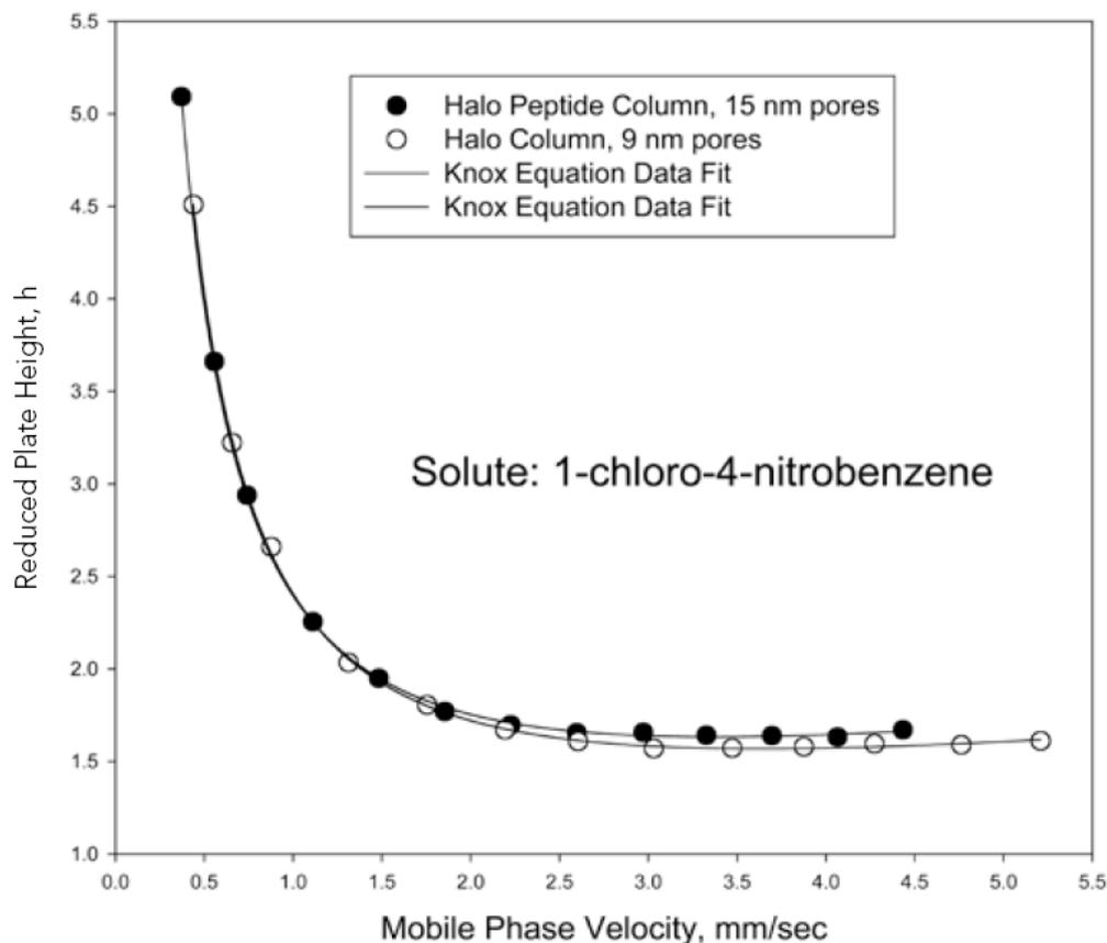
High efficiency is critical to high resolution; both particles show high peak capacity for small molecules.
