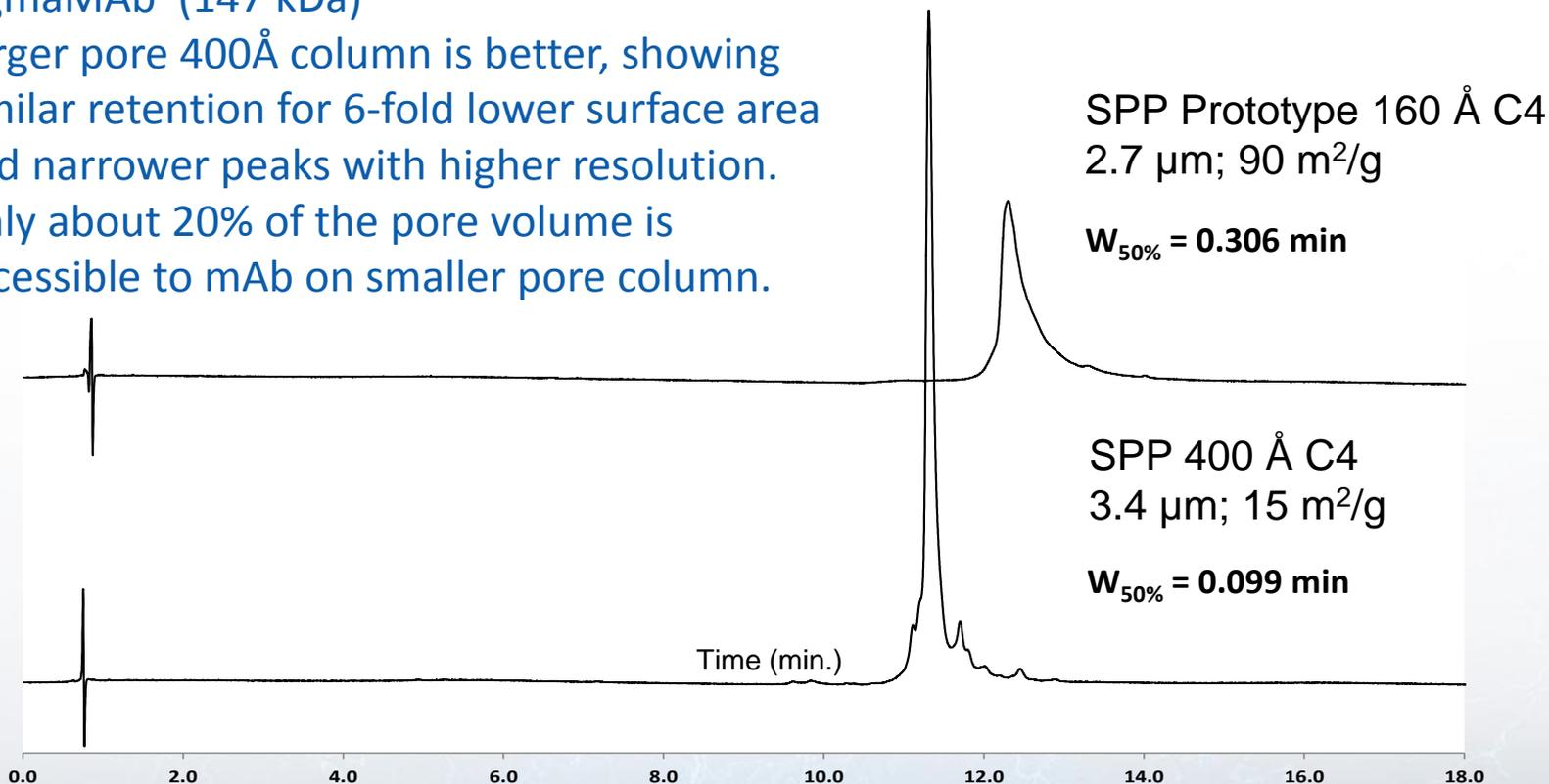
Columns: 150 mm x 2.1 mm; mobile phase: A: water/0.1% difluoroacetic acid; B: acetonitrile/0.1% difluoroacetic acid; gradient: 27-37% B in 20 min; flow rate: 0.4 mL/min; temperature: 80 °C; injection volume: 2 μL; detection: 280 nm
