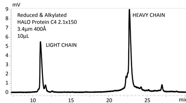
Reduced Trastuzumab 1mg/mL in 0.1%TFA, 0.2mL/min, gradient 28-34% in 40 min, 80°C, 280nm, Mobile phase A: 0.1%DFA, B: 0.1%DFA in ACN
