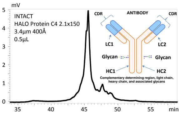
Intact Trastuzumab 2mg/mL in 0.1%TFA, 0.1mL/min, gradient 27-33%B in 80min, 80°C, 280nm. Mobile phase A: 0.1%DFA, B: 0.1%DFA in ACN
