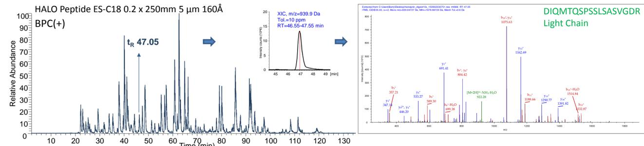
Two 250x0.2mm columns in series. Thermo Orbitrap Velos Pro/Dionex Ultimate 3000 UHPLC. 5µL injection of 3 µg/µL Trastuzumab tryptic digest. A = 0.1% DFA, B = 0.1% DFA in ACN. Loading Pump: 2%B @ 10µL/min. EXP stem cartridge 33µL HALO C4. NC Pump: 5-55%B in 182min @ 3µL/min, 60°C,
