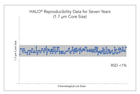
The tight control of particle size distribution shown in the following figure represents an impressive %RSD of less than 1% over the last five years highlighting the upmost quality in our manufacturing process associated to a narrow particle distribution. This result contributes greatly to our commitment for customers' long-term repeatability of separations utilizing AMT powered HPLC columns.
