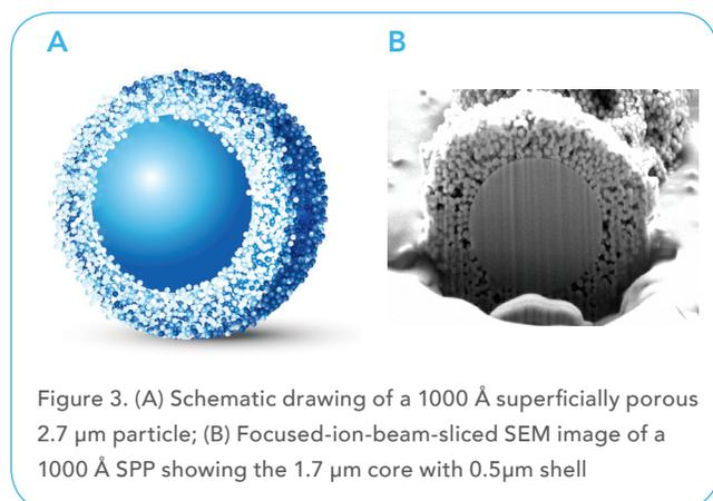
Figure 3. (A) Schematic drawing of a 1000 Å superficially porous 2.7 µm particle; (B) Focused-ion-beam-sliced SEM image of a 1000 Å SPP showing the 1.7 µm core with 0.5µm shell
